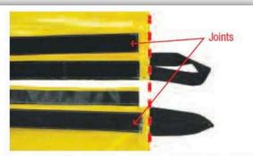
Both barriers must be aligned at the back. Make sure the joints are open.
