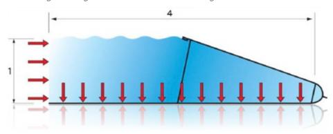
The Water-Gate anti-flood dam deploys automatically once the water begins to flow.
